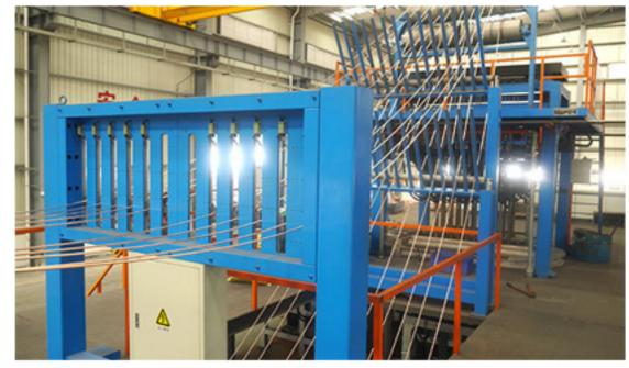
The upcasting line is used to produce the 10000~12000tons long and bright oxygen-free copper rod. This unit is also apply to produce brass rod, copper strip, copper tube and so on. That adopts energy-saving furnace, temperature control paperless recorder, Auto Alarm Function and other information management methods. And using four set of traction system to pull copper rods.
