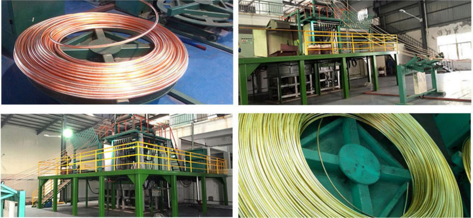
The upcasting line is used to produce the 3000~8000tons long and bright oxygen-free copper rod. This unit is also apply to produce brass rod, copper strip, copper tube and so on.That adopts energy-saving furnace, temperature control paperless recorder, Auto Alarm Function and other information management methods. The furnace is combined furnace. The size of furnace can be adjusted according to the capacity.
